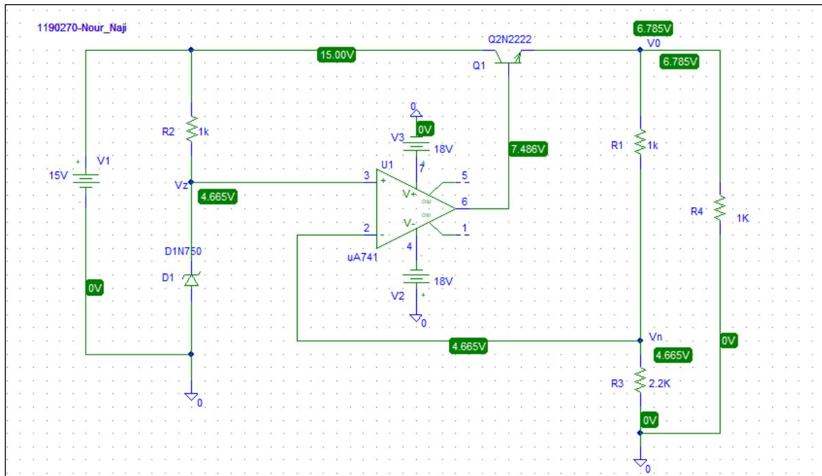
⇒ The output voltage ( $V_o$ ) = 6.785V, and the voltage across the Zener ( $V_z$ ) = 4.665 V.
