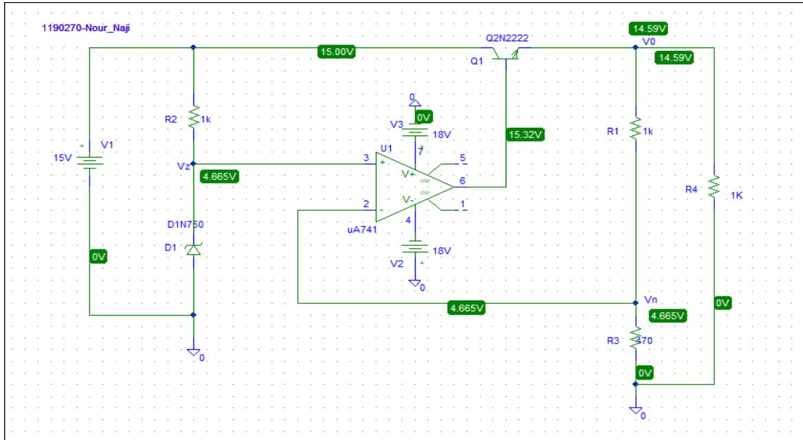
⇒ The output voltage ( $V_o$ ) = 14.59 V, and the voltage across the Zener ( $V_z$ ) = 4.665 V.
